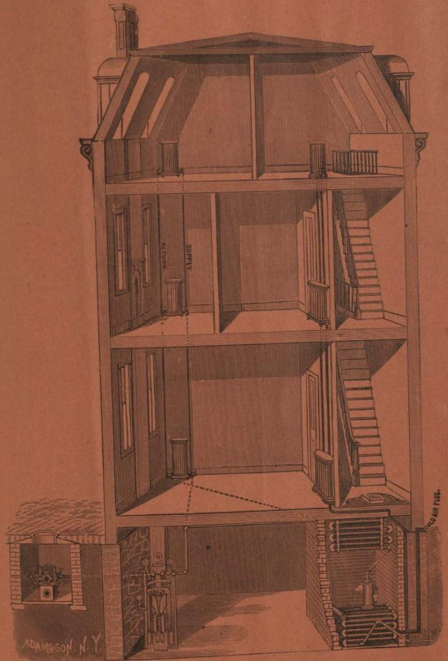
Sectional View of Building, showing course of the Steam from the Street Main to Radiators, thence to Trap and Cooling Coils in basement.
