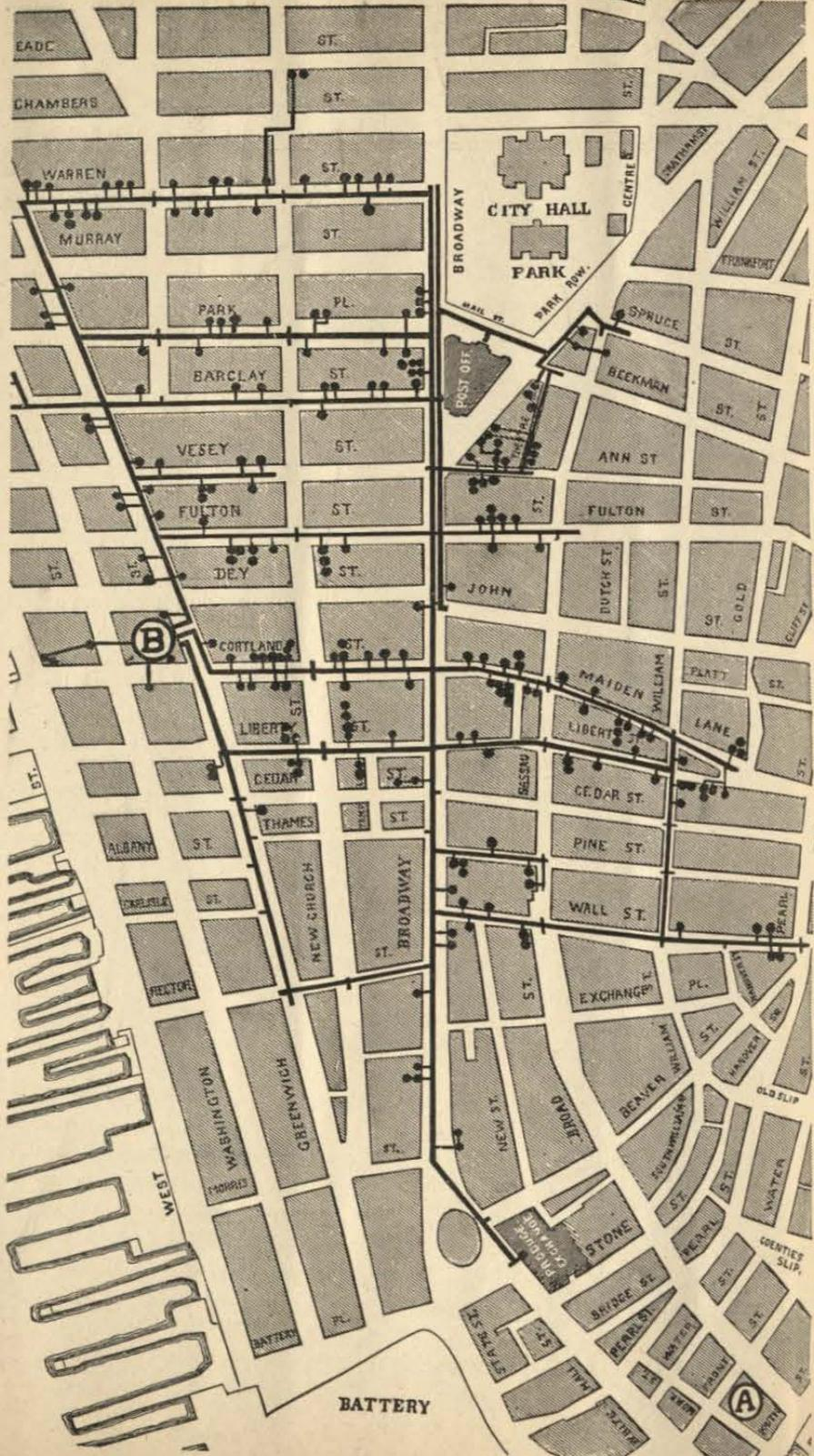
PLATE XI.—New York Steam Co., Station B, located on Greenwich St., to contain 64 Boilers, 250 Horse-Power each. Five Miles of Street Mains already in use, under constant pressure of 80 lbs.
