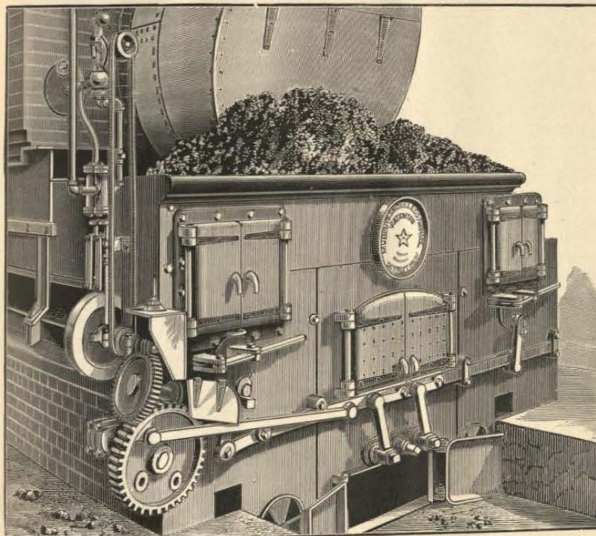
PLATE III.—Murphy Smokeless Furnace, with Automatic Feed.
