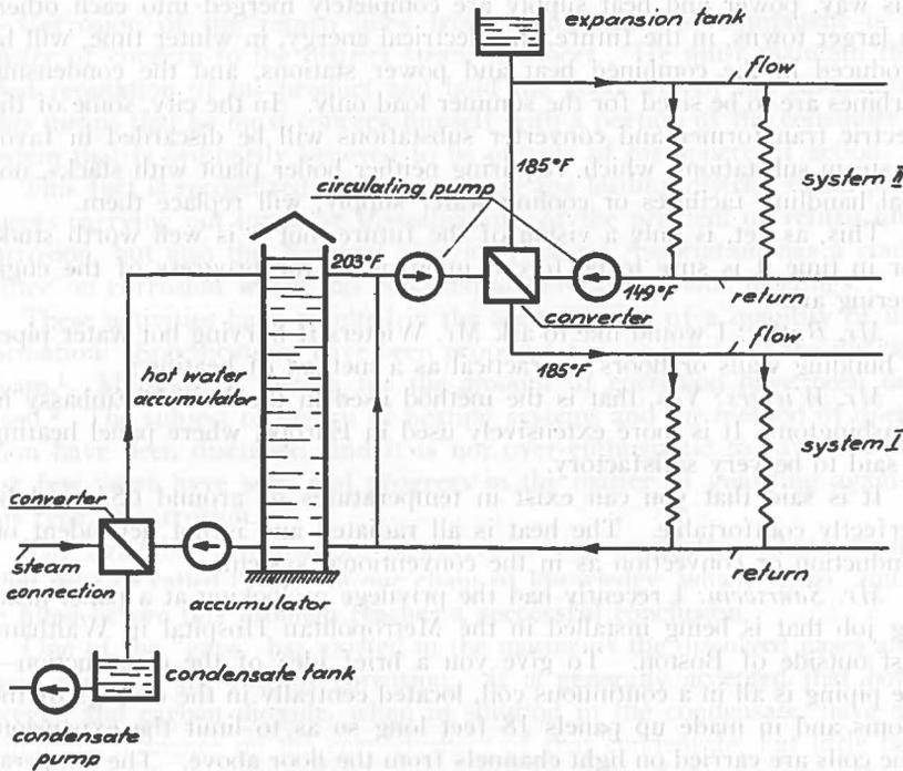
FIG. 6—Two-zone Accumulator Connections
