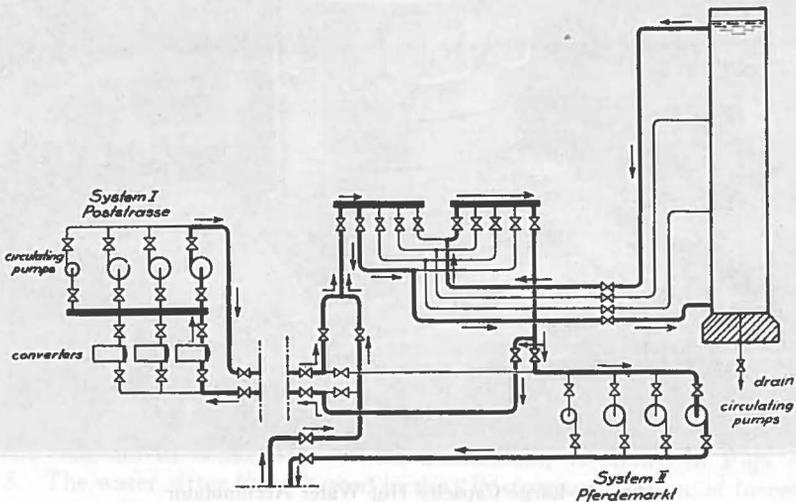
FIG. 5—Accumulator Connections
