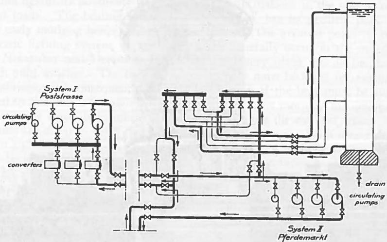
FIG. 4—Accumulator Connections
