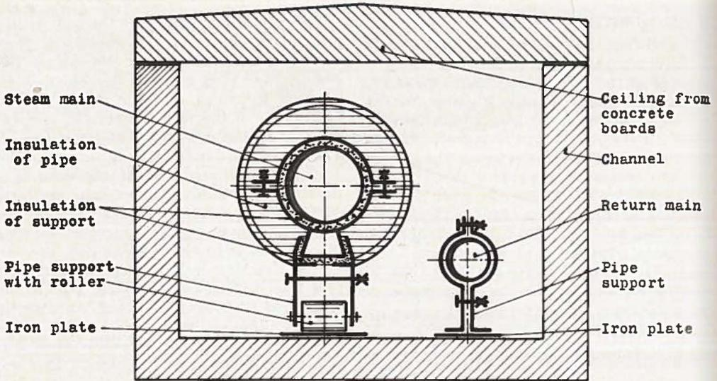
Figure 1. Cross-sectional view of a typical steam conduit.
