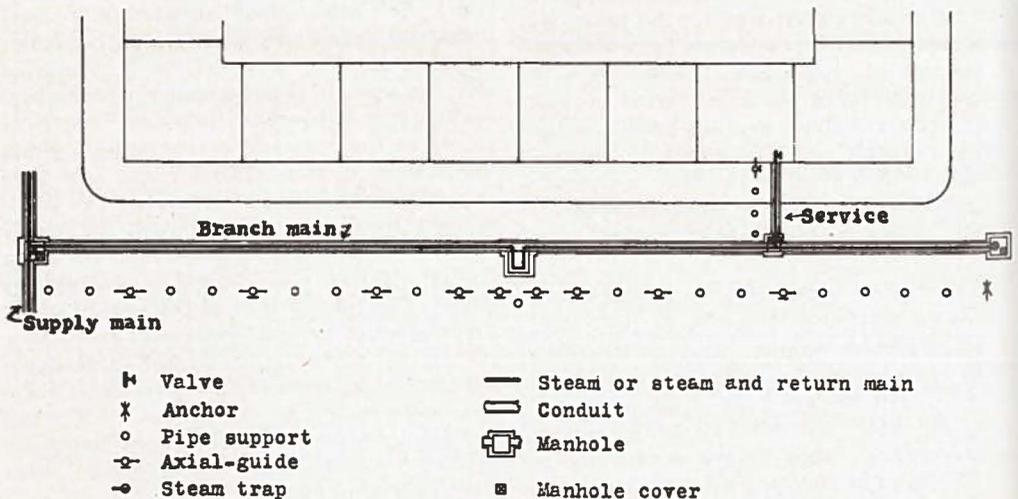
Figure 1. Typical arrangement of a branch main and service.
