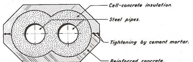
FIG. 9—Duct for Two Pipes Up to Two Inches.
