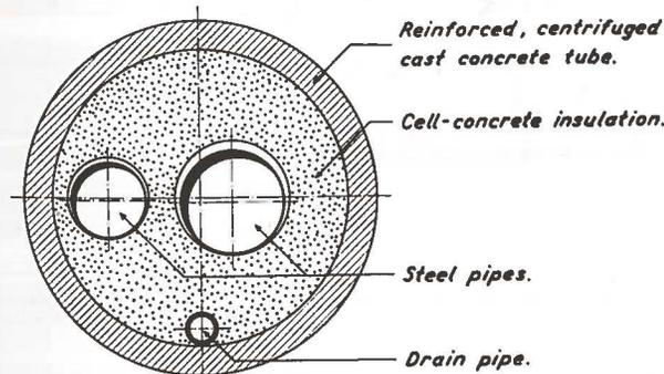
FIG. 8—Prefabricated Conduit.
