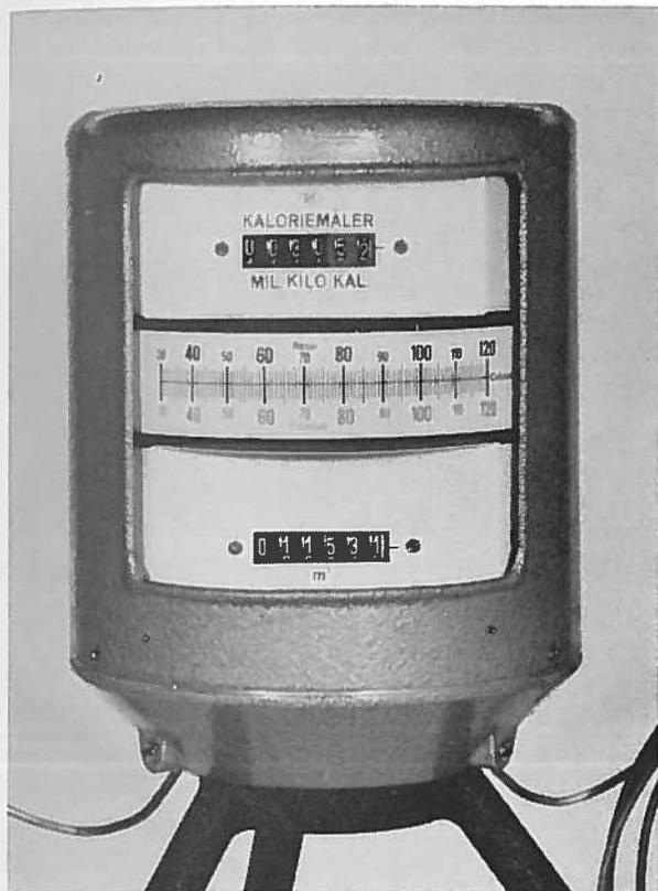
FIG. 12—Colorimeter Head for Heat Meter, Warm Water.
