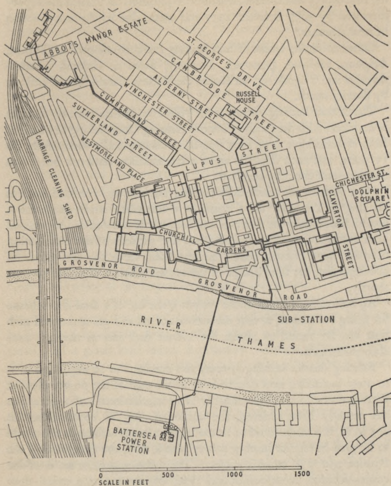
Fig. 1. THE WESTMINSTER CITY COUNCIL'S PIMLICO DISTRICT HEATING UNDERTAKING. The route of the transmission mains is shown from Battersea Power Station across the River to the sub-station. The distribution mains are also seen extending eastwards to Dolphin Square and in a north westerly direction as far as Abbot's Manor estate near Victoria Station. The heat accumulator at the sub-station is shown in Fig. 13
