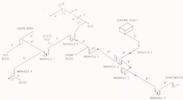
FIG. 1 — Isometric drawing of the high-temperature water system.
