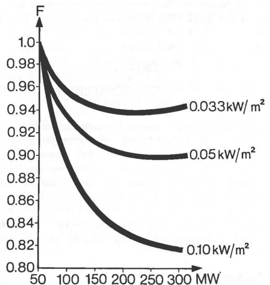
Fig. 5 — Relative specific cost of a hot water plant and a distribution network as a function of the output at different heat densities.
