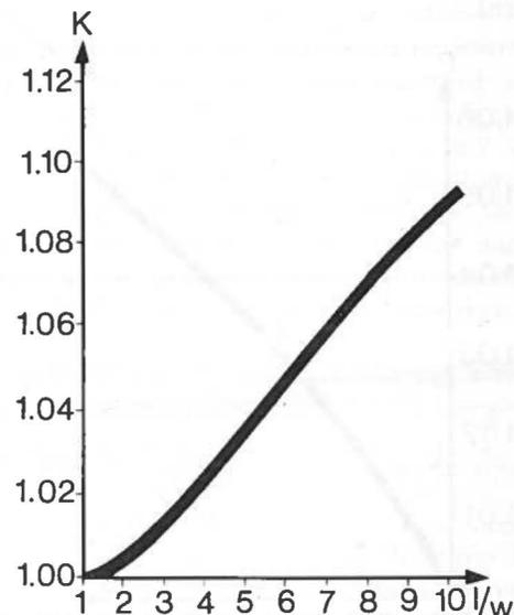
Fig. 2 — Cost of a distribution network with a varying relation of length and width for the area.
