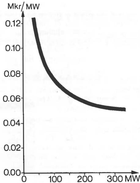
Fig. 3 — Specific cost of a hot water plant as a function of the net output.
