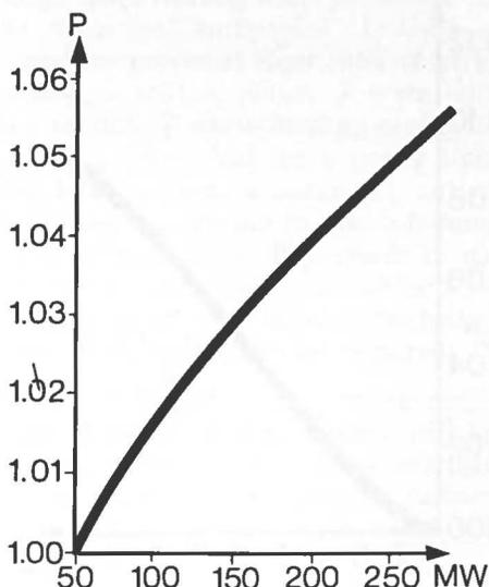
Fig. 4 — Relative specific cost of the distribution network as a function of the output.
