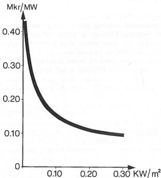
Fig. 1 — Specific cost of the distribution net as a function of the heat density of the distribution area.
