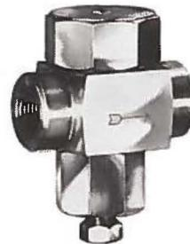
It's the D-600S thermodynamic 600 psi steam trap with a stainless steel strainer and blow-down valve built right in. Also a cylindrical perforated 20 mesh screen twice the area of any other make. Strictly from Erwel.
