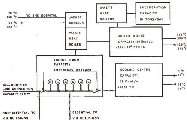
Fig. 3—Power-heat schematic diagram.
