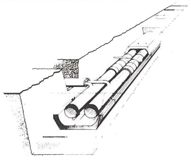
Fig. 3—Prefabricated pipeline construction: concrete duct for 700-250 mm diameter pipe; plastic covered jacket for 200-40 mm diameter.
