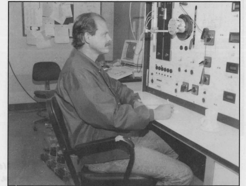
Electric Meter Test Bench
