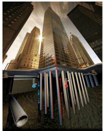
Figure 12: Geothermal Energy Piles
