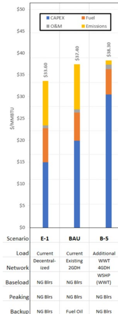
Figure 2. LCOE comparison (fossil fuel alternatives vs lowest cost electric scenario)
