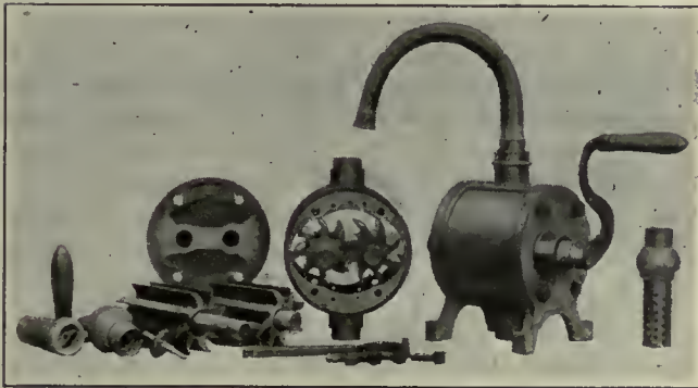
FIG. 30—ONE OF THE ORIGINAL HUBBARD PUMPS
