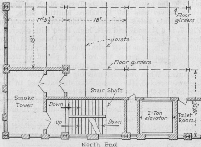
FIG. 8—SMOKE TOWER AND STAIR SHAFT
