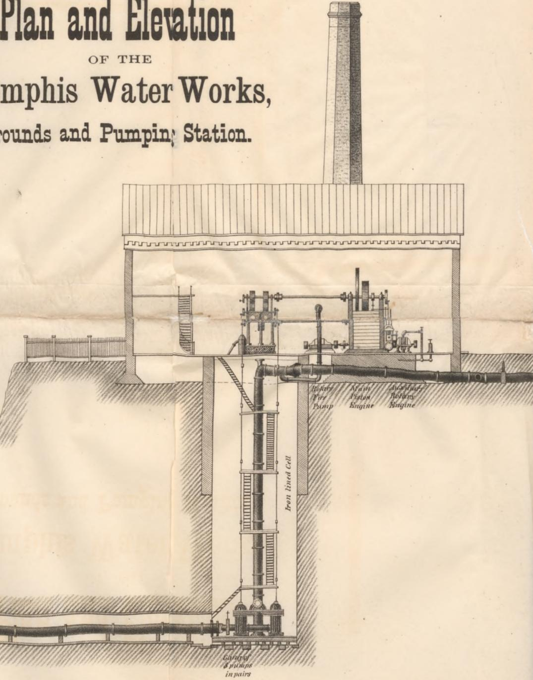
Vertical Elevation of Pumping Station, Memphis Water Works, showing outer Gravel Crib, Filter Well, Suction Main, Tunnel, Iron Well, Pumps, Machinery and Engine Building, following line A.B. in plan.
