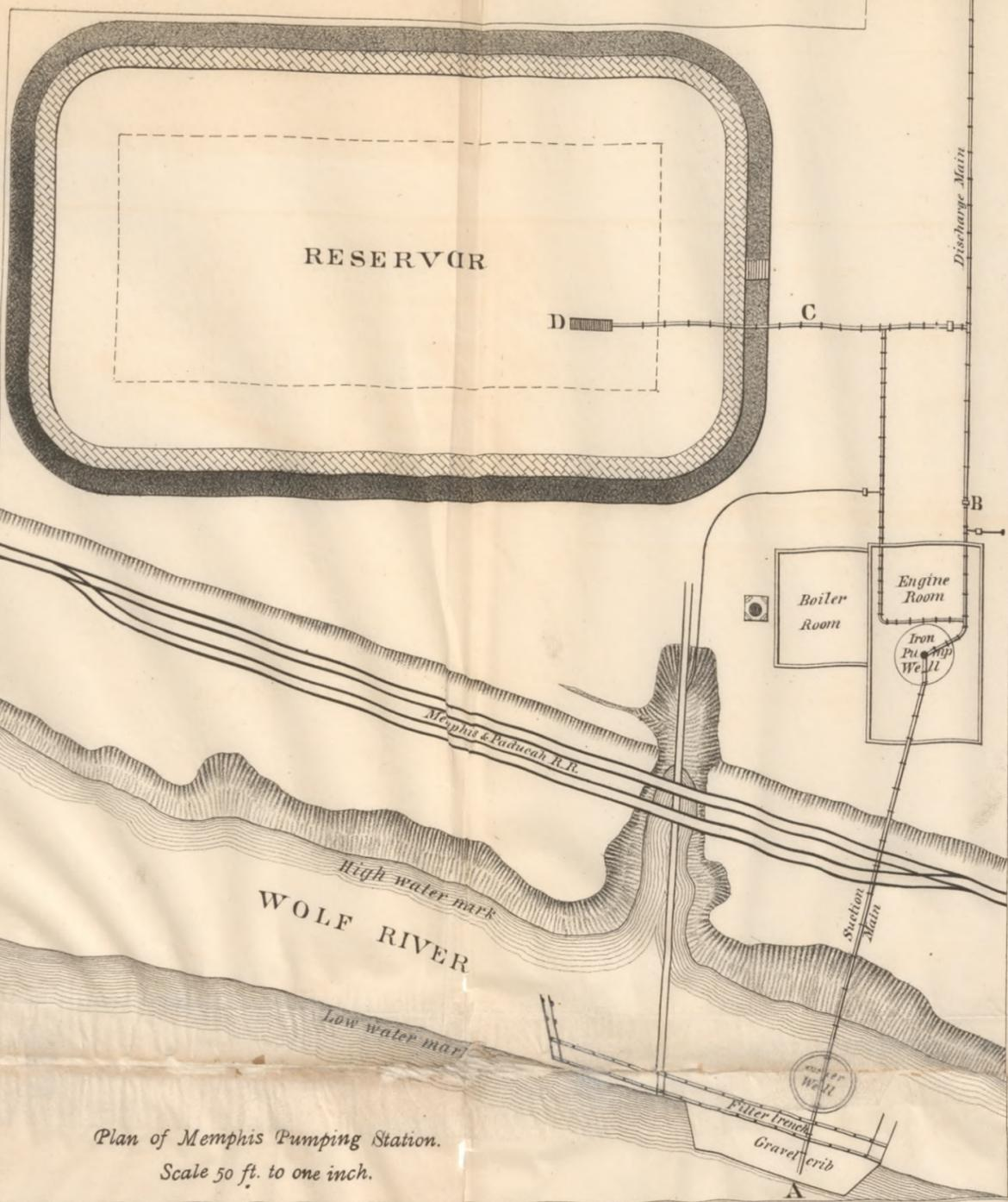
Plan of Memphis Pumping Station.
