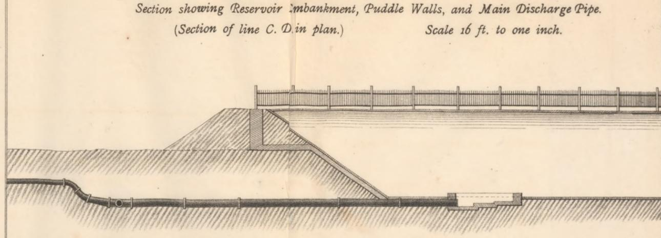
Section showing Reservoir Embankment, Puddle Walls, and Main Discharge Pipe.
