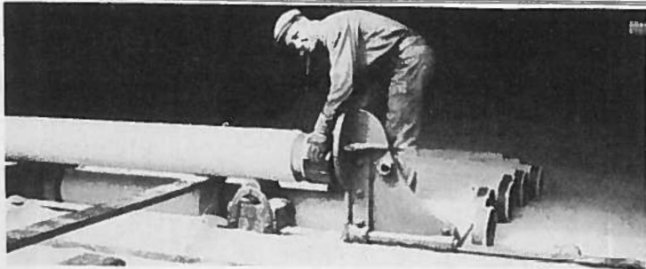
Placing Collars on Pipe at Factory
