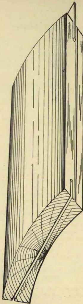
STAVE—SHOWING BUTT END, METALLIC TONGUE AND LATERAL CALKING BEAD.
